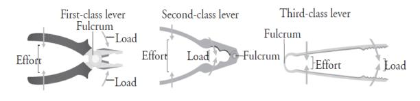
3. Simple machines are tools that make our work easier and faster by applying the force at a convenient point, which either changes the direction or the amount of force applied. There are six simple machines: lever, pulley, inclined plane, screw, wedge, and wheel and axle.
